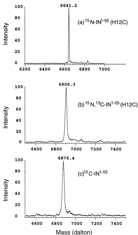
Figure 2. Mass spectra of isotopically enriched proteins: (a) <sup>15</sup>N-labeled IN<sup>1-55</sup>H12C mutant; (b) <sup>15</sup>N,<sup>13</sup>C-labeled IN<sup>1-55</sup>H12C mutant; and (c) wild-type <sup>13</sup>C-labeled IN<sup>1-55</sup>.
