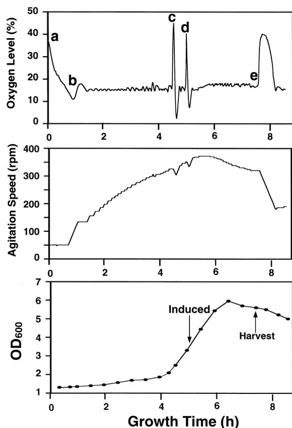
Figure 1. Oxygen level, agitation speed and OD<sub>600</sub> as a function of time for <sup>15</sup>N,<sup>13</sup>C labeling of the IN<sup>1-55</sup>H12C mutant. The time points are as follows: (a) start of run; (b) start of cell growth; (c) depletion of essential nutrients and addition of labeled nutrient (<sup>13</sup>C<sub>6</sub>-glucose); (d) depletion of essential labeled nutrient, addition of labeled nutrient (<sup>13</sup>C<sub>6</sub>-glucose) and induction; and (e) cell harvest.
