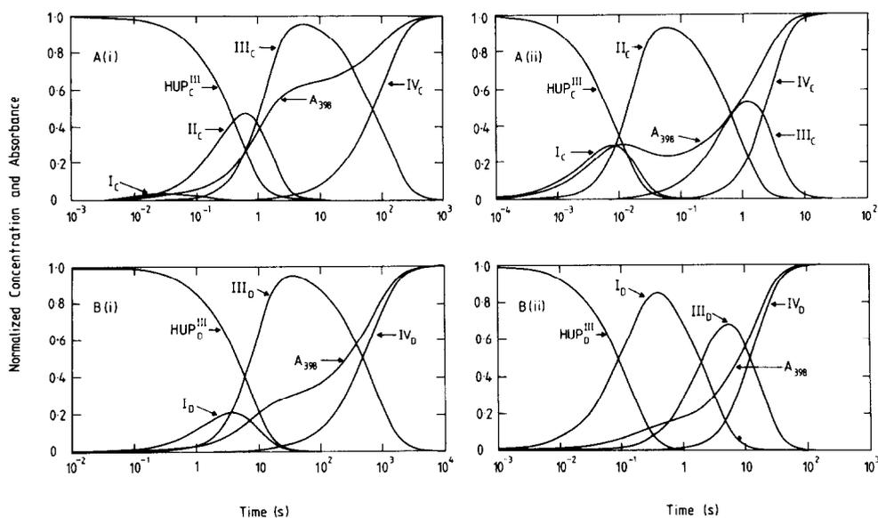
Fig. 4. Computed time courses of the concentrations of the intermediate species and absorbance changes at 398 nm in the reactions of HUP<sup>III</sup> at pH 7.0 (A), and 10.4 (B) for the schemes shown in Table II. Initial conditions: 2 μM HUP<sup>III</sup>, (i) 1 mM and (ii) 50 mM H<sub>2</sub>O<sub>2</sub>. The values of the rate constants and difference extinction coefficients (HUP<sup>III</sup> minus intermediate species) at each pH are given in Table III.
