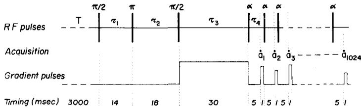
FIG. 1. Pulse sequence used to excite and detect zero-quantum frequencies. Transverse nuclear magnetization was sampled at the points indicated by  $a_1, a_2, \dots, a_{1024}$ ; immediately after each sample, the transverse magnetization was dispersed by a gradient pulse of random amplitude. The intervals  $T, \tau_1, \tau_2, \tau_3$ , and  $\tau_4$  were chosen as described in the text.
