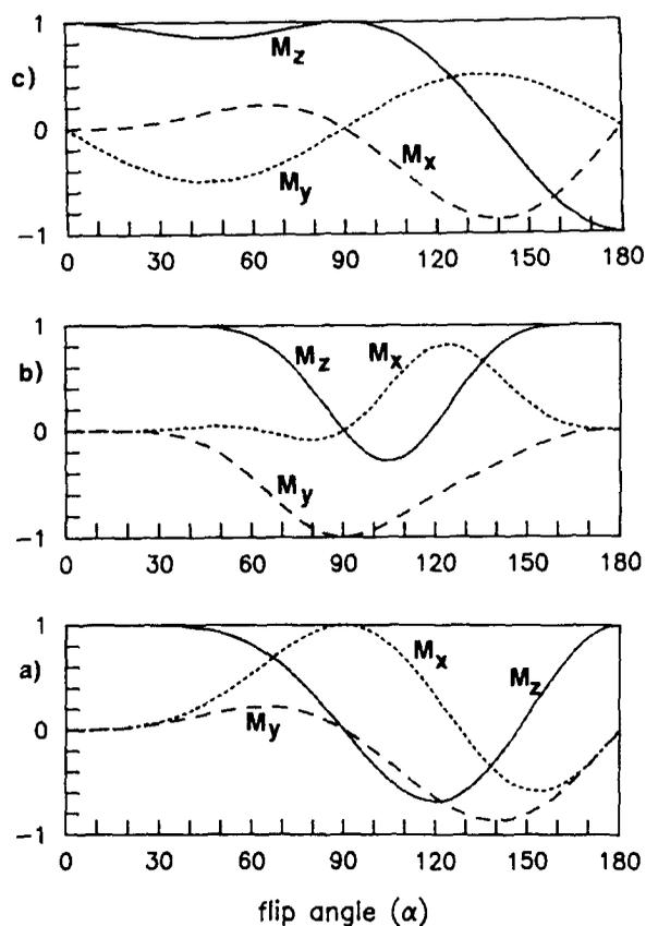
FIG. 1. The effect of the composite pulses (a) I, (b) II, and (c) III on a magnetization vector of unit intensity that is initially aligned along the z axis. The flip angle,  $\alpha$ , represents the flip angle of each individual pulse within the composite pulse unit.
