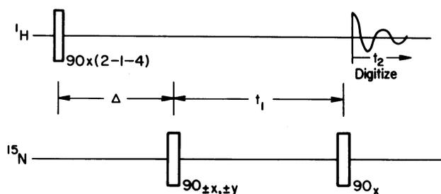
FIG. 1. Pulse sequence used for multiple quantum 2D  $^1\text{H}$ — $^{15}\text{N}$  NMR.  $^1\text{H}$ — $^{15}\text{N}$  decoupling can be accomplished by introducing a second delay  $\Delta$  following the second  $90^\circ$  nitrogen pulse and irradiating  $^{15}\text{N}$  during  $t_2$ .
