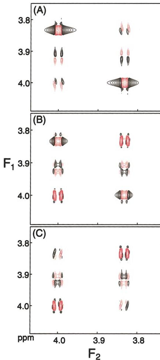
**FIG. 3.** Simulated 2D CT-COSY spectra, showing the artifactual resonances between two strongly coupled spins *A* and *B*, which have a chemical shift difference  $\delta = 100$  Hz and scalar coupling  $J_{AB} = 10$  Hz, at different constant-time delays of (A) 150, (B) 110, and (C) 100 ms.
