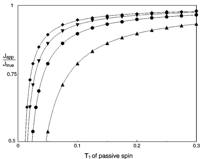
**FIG. 5.** The ratio of the apparent  $J_{AX}$  coupling ( $J_{app}$ ) over the true coupling ( $J_{true}$ ) derived using JINX of the  $A \rightarrow M$  cross peak in an  $AMX$  spin system, as a function of the  $T_1$  of spin  $X$ . The  $J_{app}/J_{true}$  ratio is calculated for  $J_{true}$  values of 5 (▲), 10 (●), 15 (▼), and 20 Hz (◆), assuming  $T_2^A = 100$  ms,  $T_1^M = 200$  ms, and  $J_{AM} = 4$  Hz.
