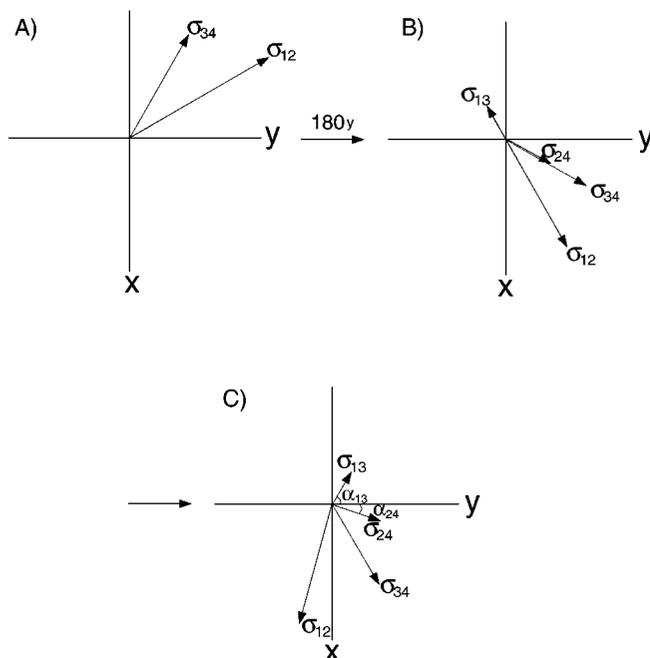
**FIG. 2.** Evolution of coherences  $\sigma_{12}$  and  $\sigma_{34}$  during the CT-COSY experiment. (A) Just prior to the moving  $180^\circ$  pulse; (B) just after the  $180^\circ$  pulse, when part of the  $\sigma_{12}$  and  $\sigma_{34}$  coherences has been transferred to  $\sigma_{24}$  and  $\sigma_{13}$ ; (C) immediately prior to the final  $90^\circ$  pulse.
