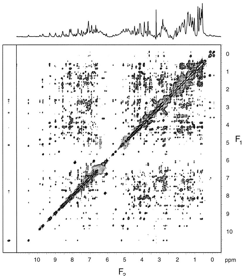
Fig. 3. 600 MHz 2D NOESY spectrum of 3 mg BPTI, detergent-solubilized (40 mg perfluorinated surfactant) in 5  $\mu\text{l}$  H<sub>2</sub>O, 30  $\mu\text{l}$  TFE, and CO<sub>2</sub>, to a final total volume of 0.4 ml. On the left, a narrow F<sub>1</sub> strip from the NOESY spectrum in H<sub>2</sub>O is shown, taken at the chemical shift of the most downfield shifted amide proton (Tyr<sup>23</sup>).
