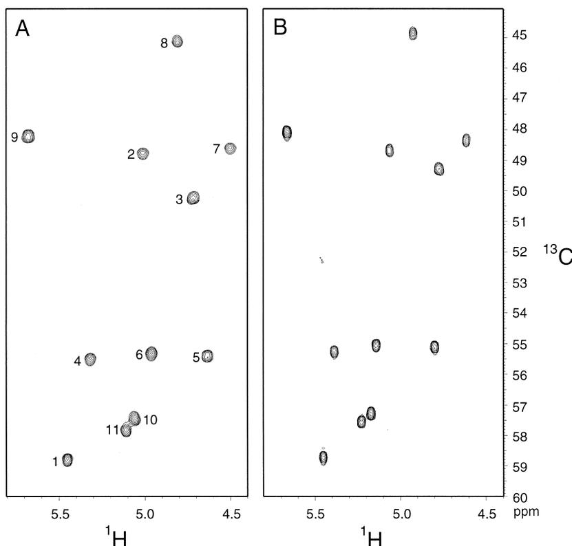
Fig. 1.  $^1\text{H}$ - $^{13}\text{C}$  region of the  $^{13}\text{C}$ - $^1\text{H}$  HSQC spectra of cyclosporin A, recorded in (A)  $\text{CDCl}_3$  and (B) in a 7:1 mixture of  $\text{CO}_2$  and  $\text{CD}_3\text{OD}$ . Spectra have been recorded at 600 MHz,  $20^\circ\text{C}$ . Numbers in (A) correspond to the residue position in the peptide (see Table 1).
