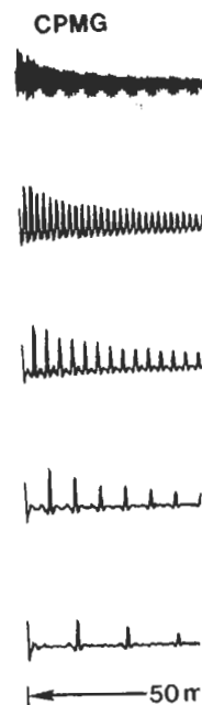
FIG. 5. Echo trains during a Meiboom-Gill (CPMG) sequence. Initial magnetization. In the CPMG phase of the initial magnetization sequence pulse imperfections cause the CPMG sequence pulse errors in
